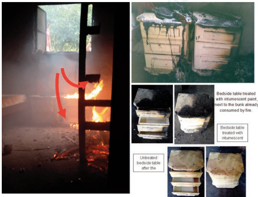
Figure 5. Air column formed between the window and the door, keeping the flames to one side.
