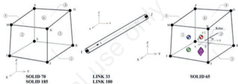
Figure 2. Finite elements used to build the three-dimensional model of partially encased columns.
