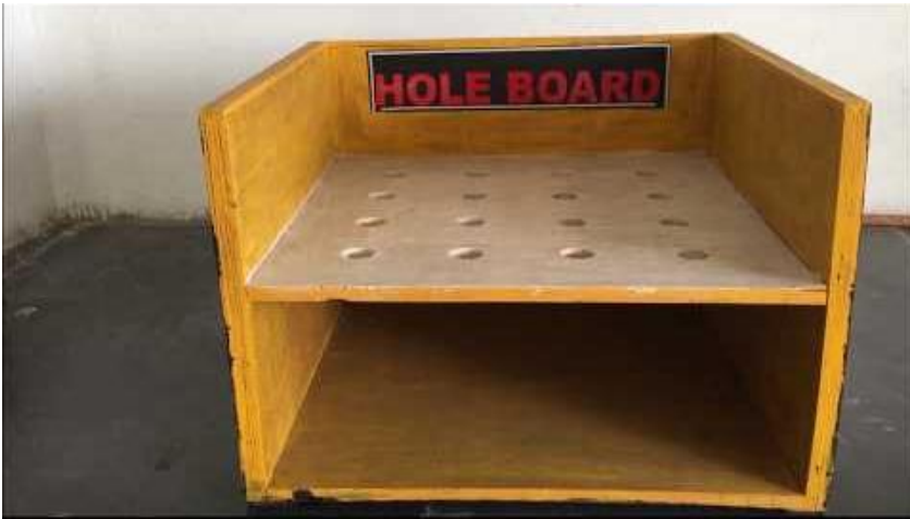
Supplementary Figure 3. Hole Board Test apparatus used in anxiolytic activity.
