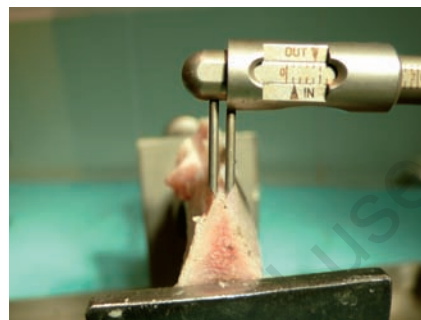
Figure 10. Experimental setup for TKW-CS-Tips testing with selected cow-rib's crest-widths of 1 to 1.5 mm.
