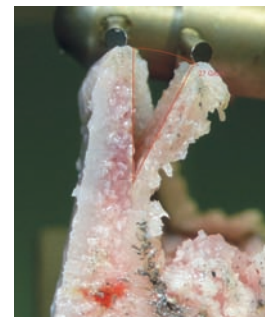
Figure 8. Mean widening angle at 8 mm osteotomy depth and 4 mm widening gap. No cracks at the baseline can be detected.
