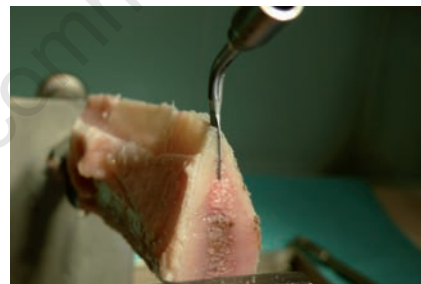
Figure 11. Cutting profile of the ultrasonic TKW-CS1 tip (lossless bone cut).
