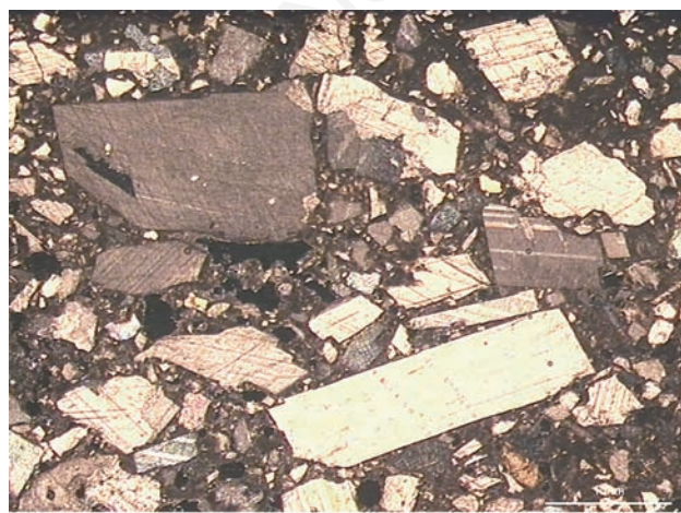
Figure 4. Cividate-a, Palazzo street, 1 st century [thin-section, cross-polarised light (XPL)]. Finish coat: aggregate made of crushed calcite crystals.
