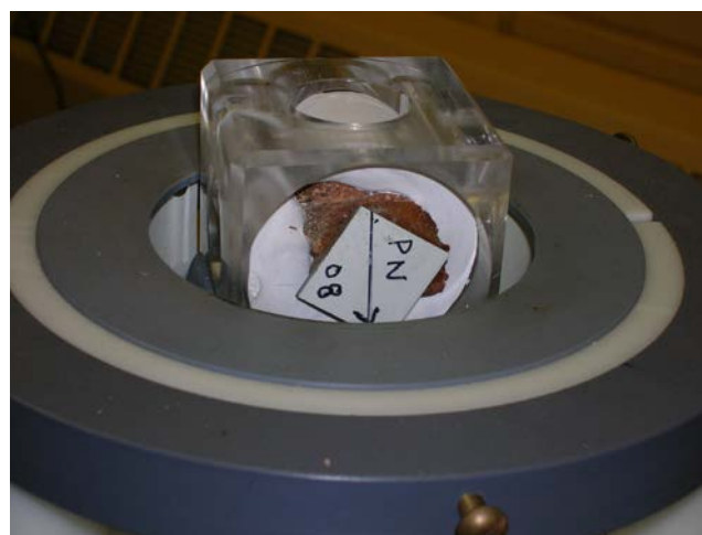
Figure 4. A typical sample being lowered into the cylindrical magnetic shield of the Molspin spinner magnetometer. The plastic square measures 2×2cm.
